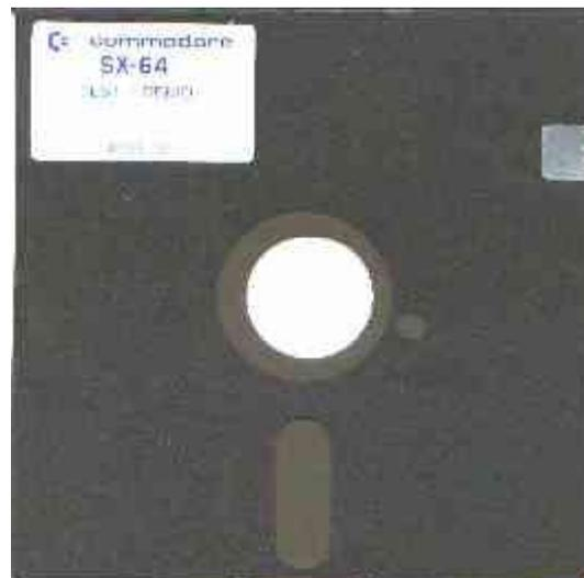
If you flip the disk, the index hole is in the wrong position, and the drive cannot tell wether the disk is spinning or not. Since there are no index pulses, the drive assumes that the disk is not spinning, and therefore the data lines to the Catweasel controller are disabled. The problem why you cannot read the reverse sides is not located in the Catweasel controller, but in the 5,25 inch drive. Some hardware patching is necessary to work around this.
