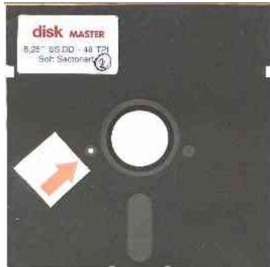
The normal disks (the following picture shows the SX-64 test/demo disk) only have one index hole.
