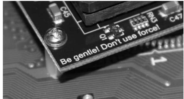
The screws also make additional electrical contact. This is desired! It is not required to insulate the screws.
